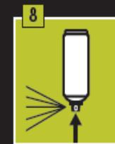
Clean the valve by turning can upside down and spraying until only propellant leaves the nozzle.
