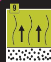
Allow 1st coat to flash off for 20 mins and apply a 2nd coat. Repeat step 8.
