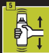
Dispose of the red button (to identify activated aerosols) and shake for two minutes. Once activated use within 60 minutes (@ 68°F).
