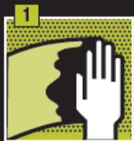
Clean and degrease surface. Abrade the surface with P80-P120 grit sand paper. Reclean.
