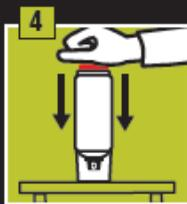
Place can on stable, horizontal surface and apply even vertical pressure on red button to activate.
