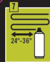
First test the spray, hold the can approximately 24"-36" from the object and apply the first coat with a steady even motion.
